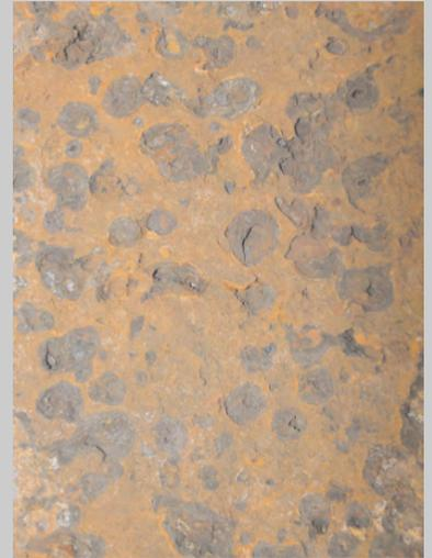
Localised corrosion for high levels of salt
